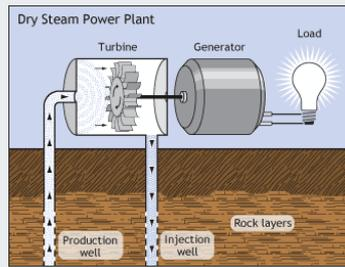
Figure 2: Direct dry steam plant (Source: U.S. Department of Energy, Energy Efficiency & Renewable Energy (public domain))
