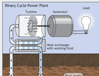
Figure 4: Binary cycle power plant (Source: same as above)
