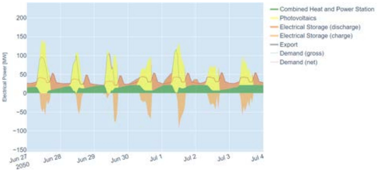
Figure 31: Time series for one week in June for electricity supply and demand for the scenario with no wind power installed
