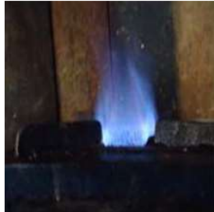
Optimal burning—blue flame
