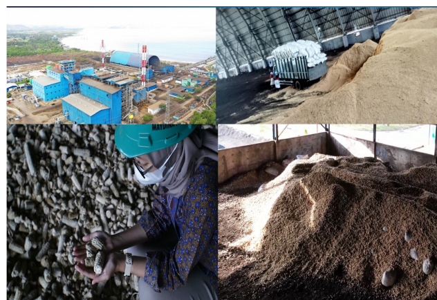
Figure 3. Co-firing initiative at two coal power plants in WNT Province, with biomass comprising 10-50% of the daily fuel mix (Photo source: WNT Energy Agency)
